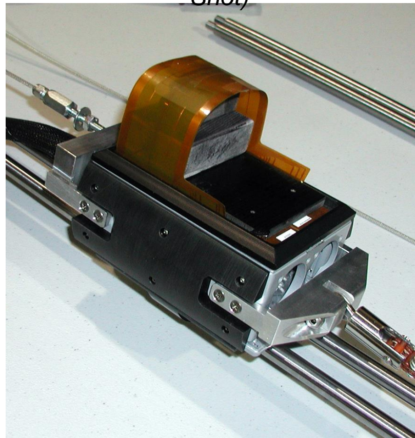
Adapted MWM-Array Probe (Angle Shot)
